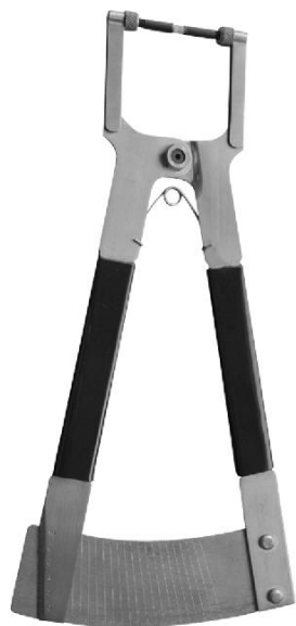
MI-011 Wide Throat Lens Thickness Gauge Accommodates Lens Blanks Of Over 90mm Diameter & 22mm in Thickness. 47mm Throat Depth, 0.1mm Graduations. Overall Length 9-3/4"
