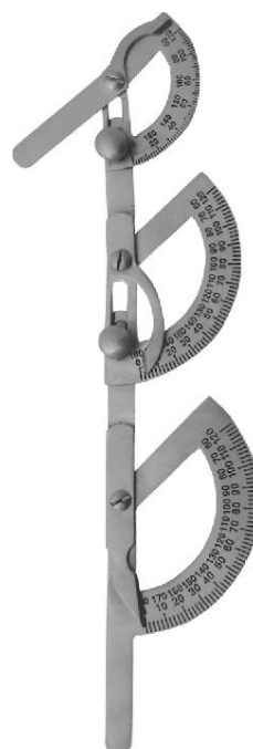
MI-04 Finger Goniometer 3 Joint Measuring Range 180°
