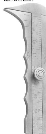
MI-05 Carroll Pocket Goniometer 6" Long With 180° Scale In 5° Increments. Fixed Leg Has 5" Linear Scale Calibrated In Inches & Centimeter
