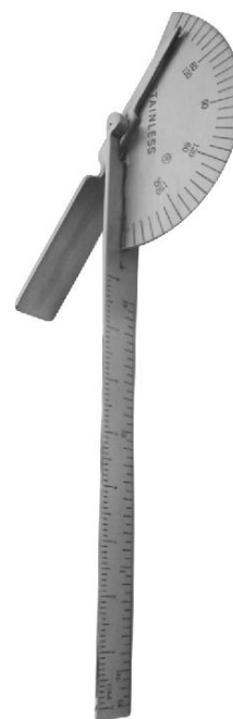
MI-05 Carroll Pocket Goniometer 6" Long With 180° Scale In 5° Increments. Fixed Leg Has 5" Linear Scale Calibrated In Inches & Centimeter
